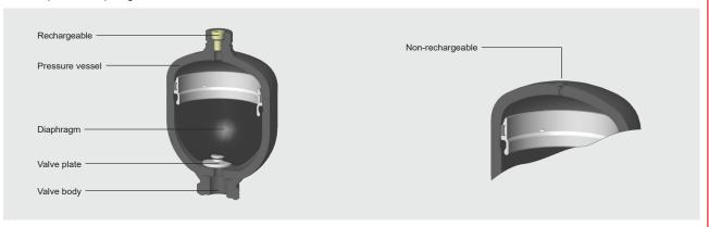
HYDAC screw type diaphragm accumulators consist of the following key individual components:
